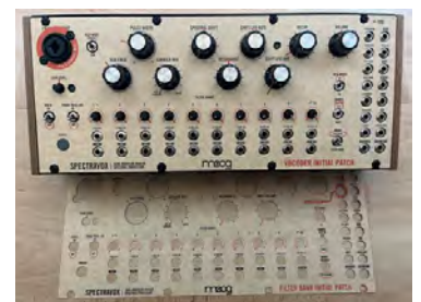
Spectravox is purely analog and cannot be saved, but overlays make it easier to get started.
